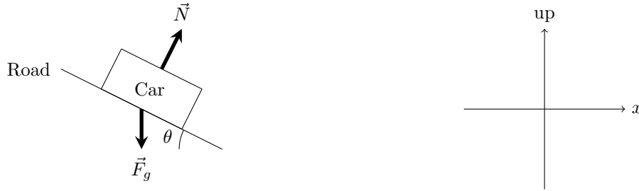
Figure 41: We can tilt the road so that the normal force has an x -component pointing along the x -direction toward the center of the circle.
