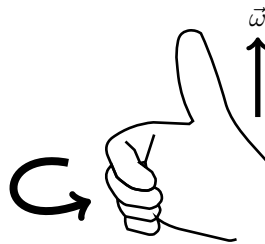
Figure 53: The right hand rule: curl the fingers of your right hand in the direction of rotation as shown. Then your thumb points in the direction of \vec{\omega} .
